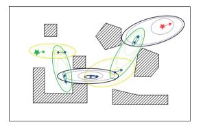
It is possible to guarantee that a path is feasible given the uncertain dynamics of robot, constraints and obstacles in the cluttered scenario.
